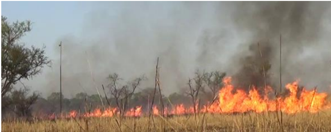
Figure 6: An experimental fire in Comoé National Park, Côte d'Ivoire is observed by radiometers mounted on six meter poles to measure the heat release of the fire in a similar manner as a satellite does.
